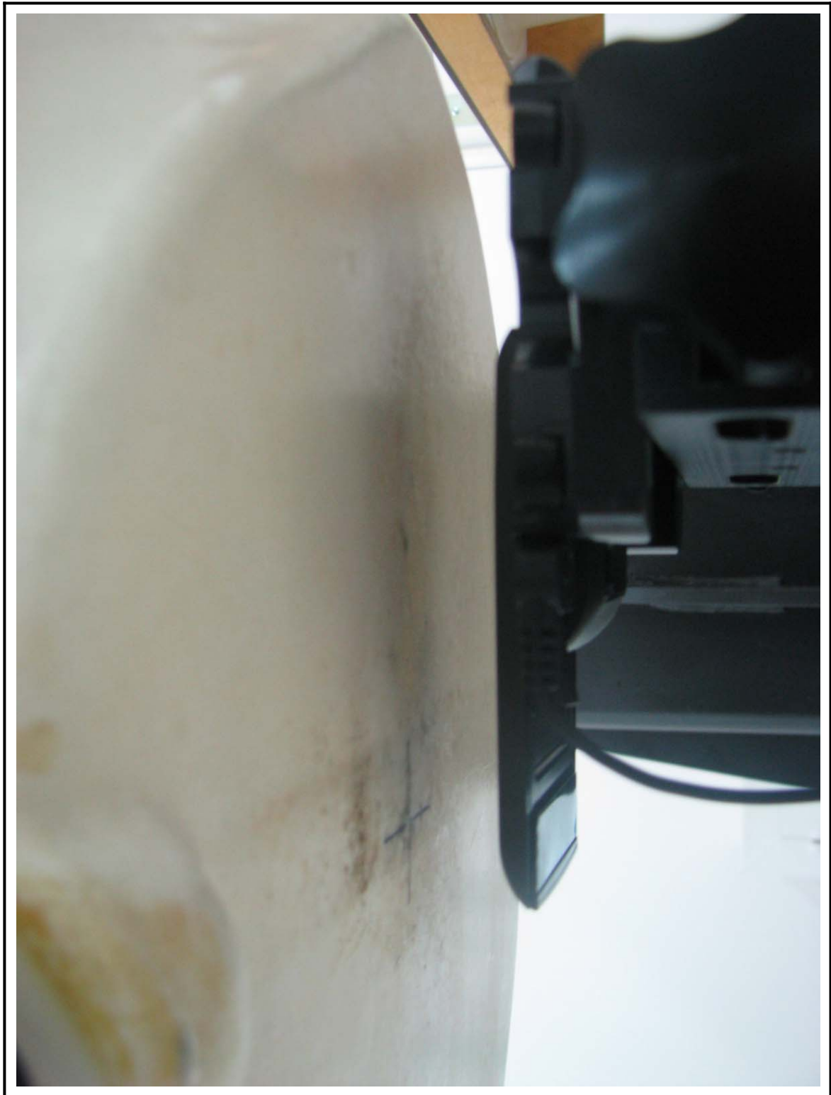
Figure 10 Body SAR Test Setup – w/o Holster
