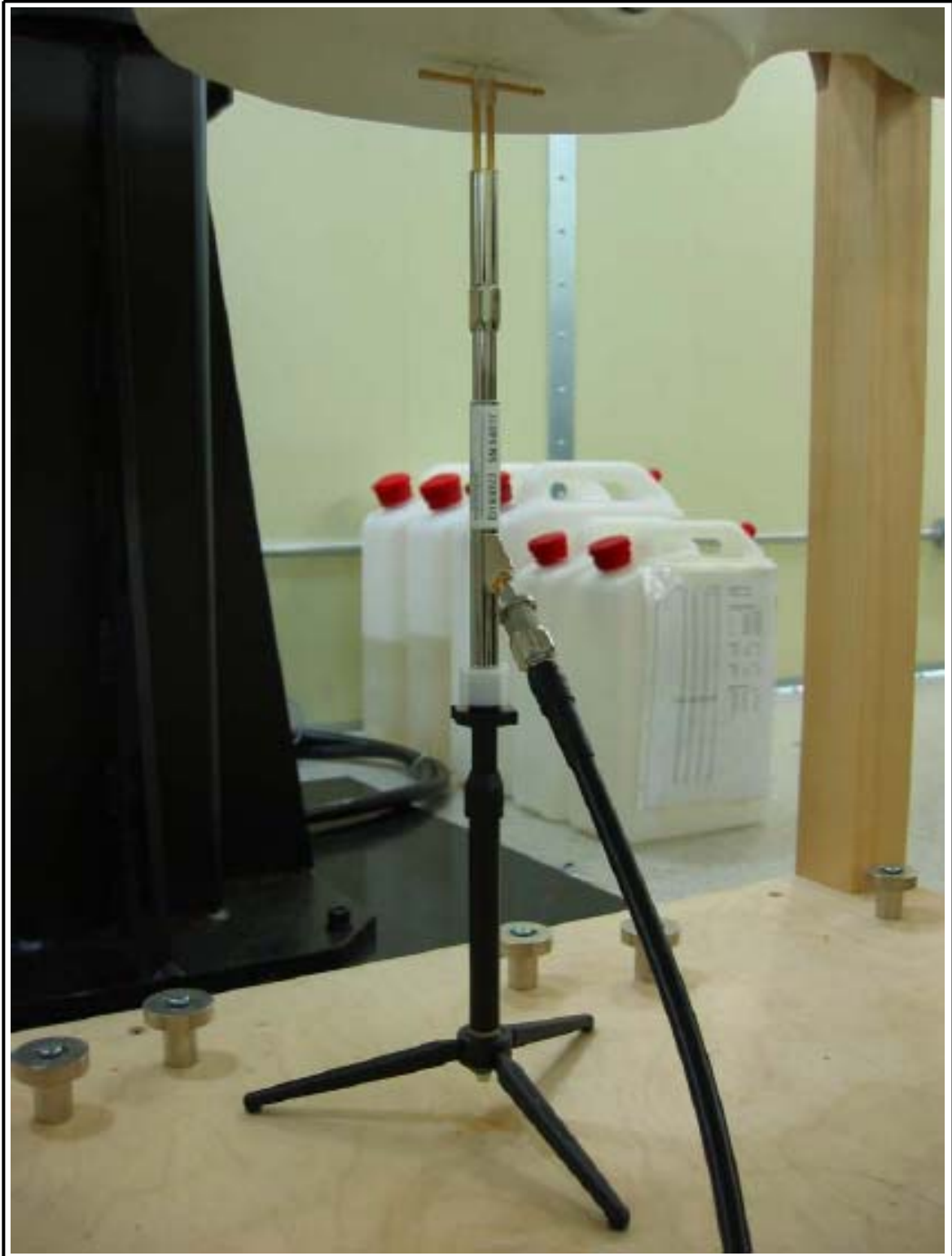
Figure 2 1900 MHz Dipole Validation Test Setup
