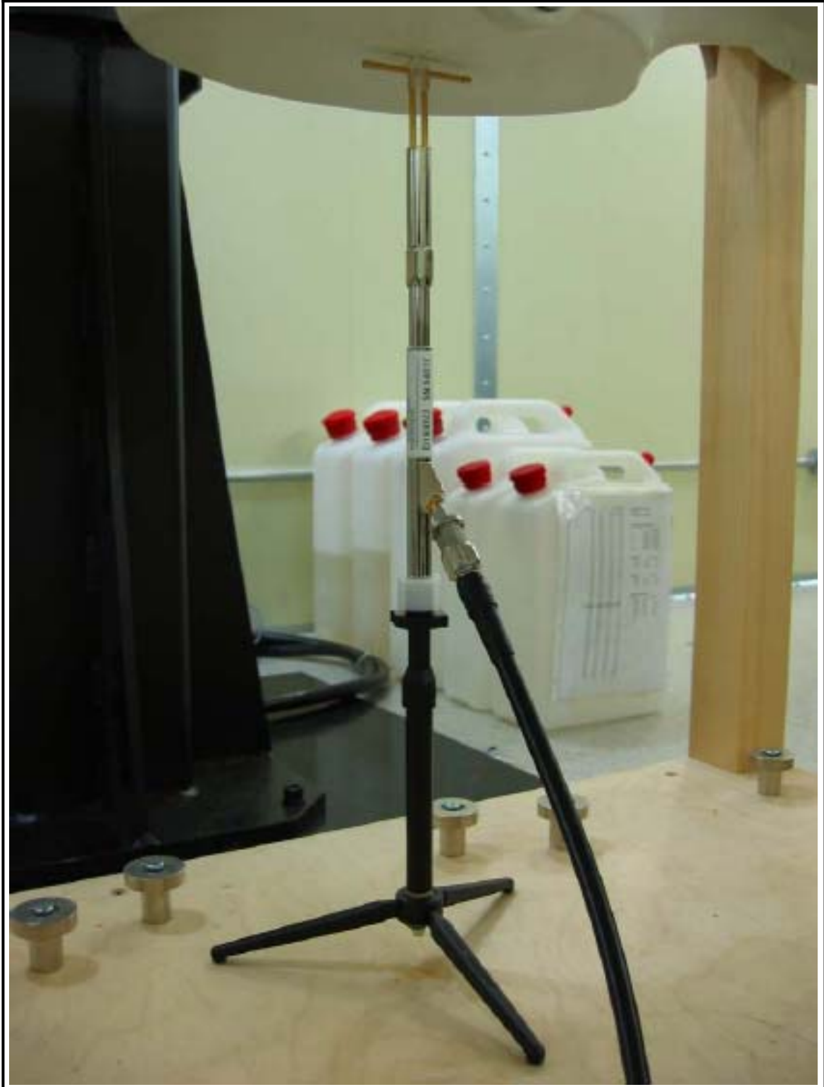
Figure 2 1900 MHz Dipole Validation Test Setup
