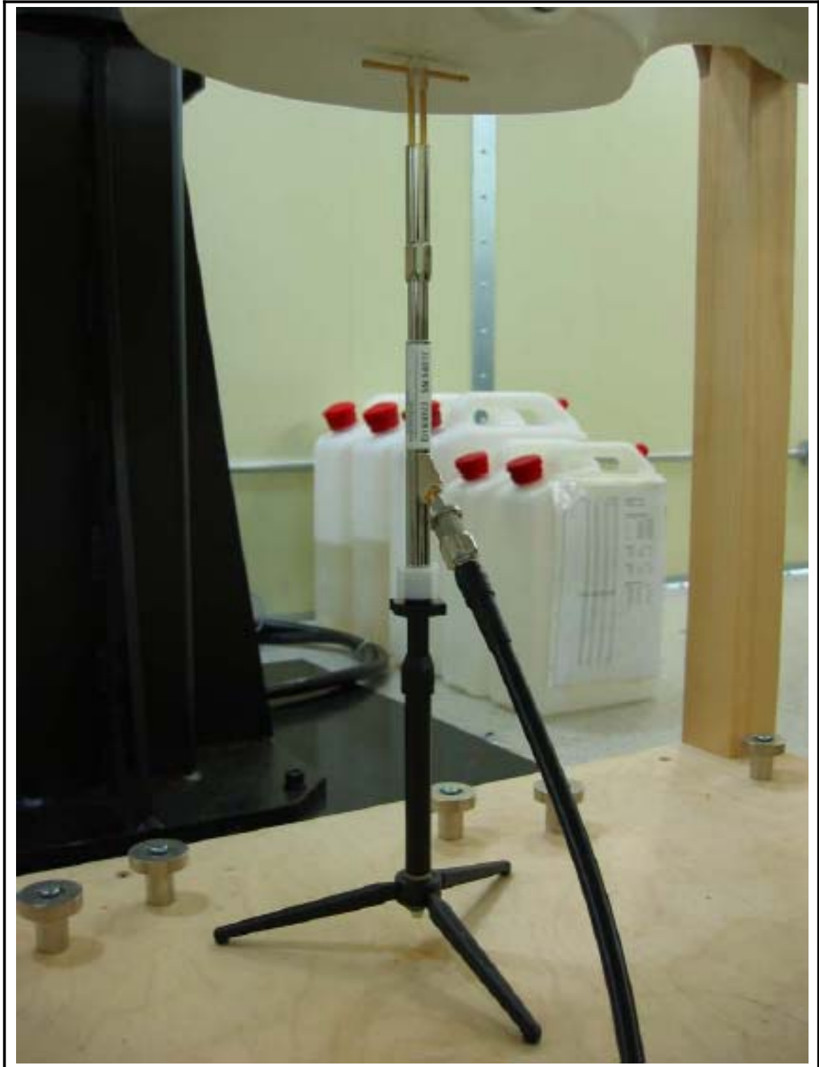
Figure 2 1900 MHz Dipole Validation Test Setup
