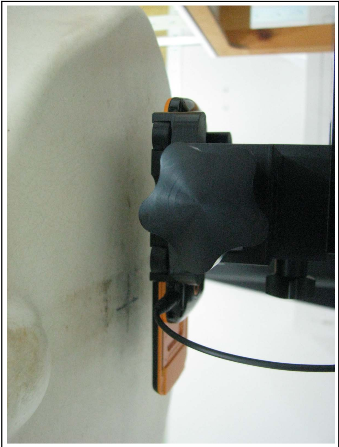
Figure 10 Body SAR Test Setup – w/o Holster
