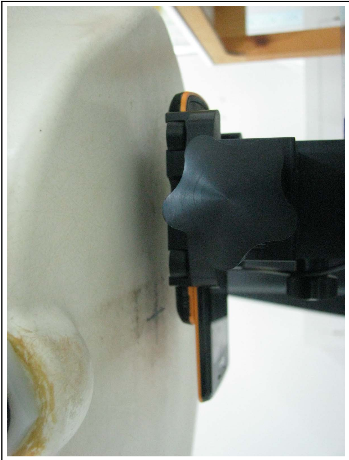
Figure 11 Body SAR Test Setup – w/o Holster
