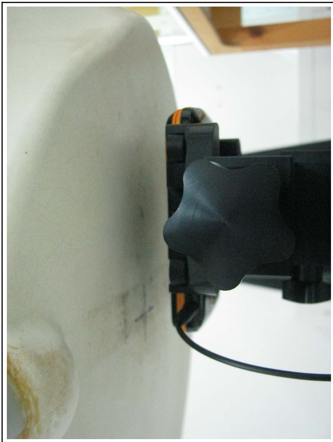
Figure 9 Body SAR Test Setup – w/o Holster
