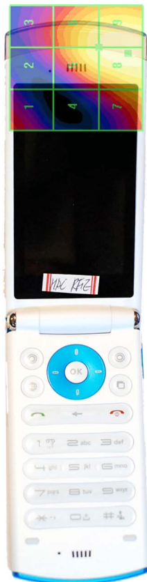
Figure 17-4 E-Field WD Scan overlay
