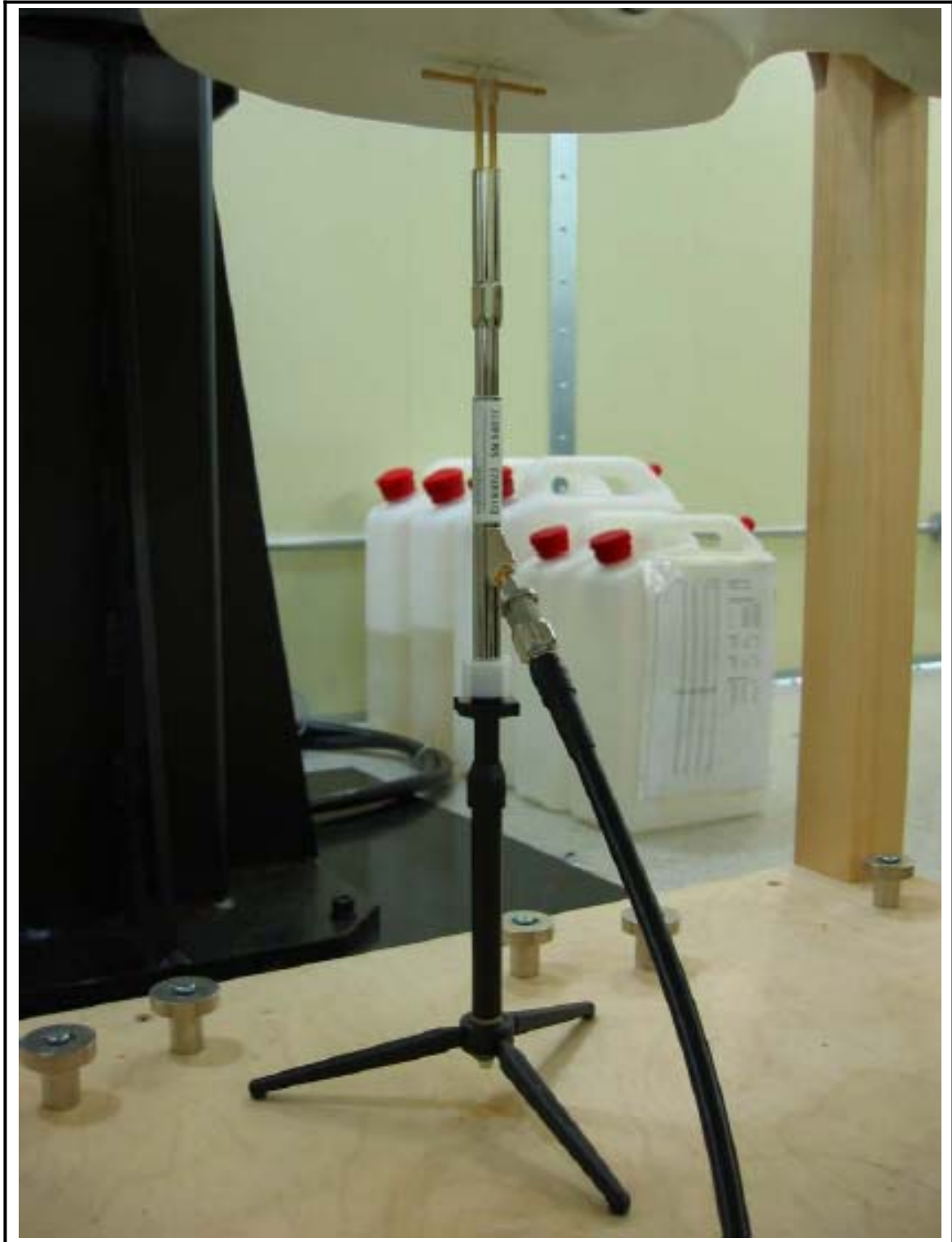
Figure 1 1900 MHz Dipole Validation Test Setup
