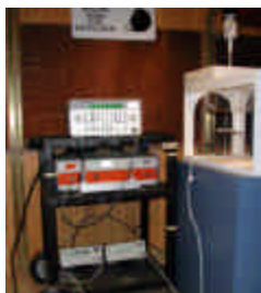
Figure A.0 Dipole Validation Test Setup
