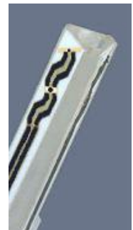
Figure 3.2 Probe Thick-Film Technique
