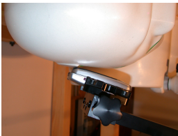
Figure 14.2 Right Head SAR Test Setup -- Ear / Tilt Position – Slide In--
