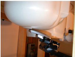
Figure 14.2 Right Head SAR Test Setup -- Ear / Tilt Position – Slide Out--
