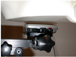
Figure 14.5 Body SAR Test Setup -- w/o Belt-clip – Slide In --
