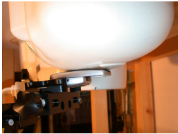
Figure 14.3 Left Head SAR Test Setup -- Cheek / Touch Position – Slide Out --
