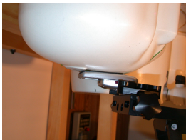
Figure 14.1 Right Head SAR Test Setup -- Cheek / Touch Position -- Slide Out --
