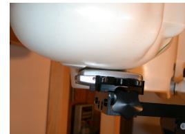
Figure 14.1 Right Head SAR Test Setup -- Cheek / Touch Position -- Slide In--
