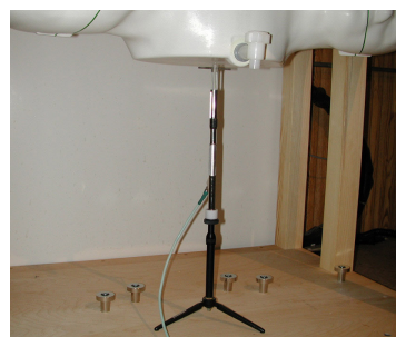
Figure 12.1 Dipole Validation Test Setup
