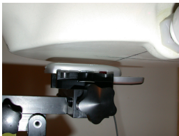
Figure 14.5 Body SAR Test Setup -- w/o Belt-clip – Slide Out --
