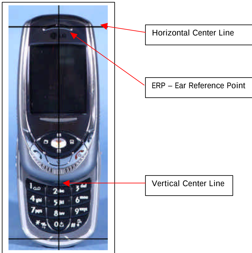
Figure 12.1 Handset Reference Points
