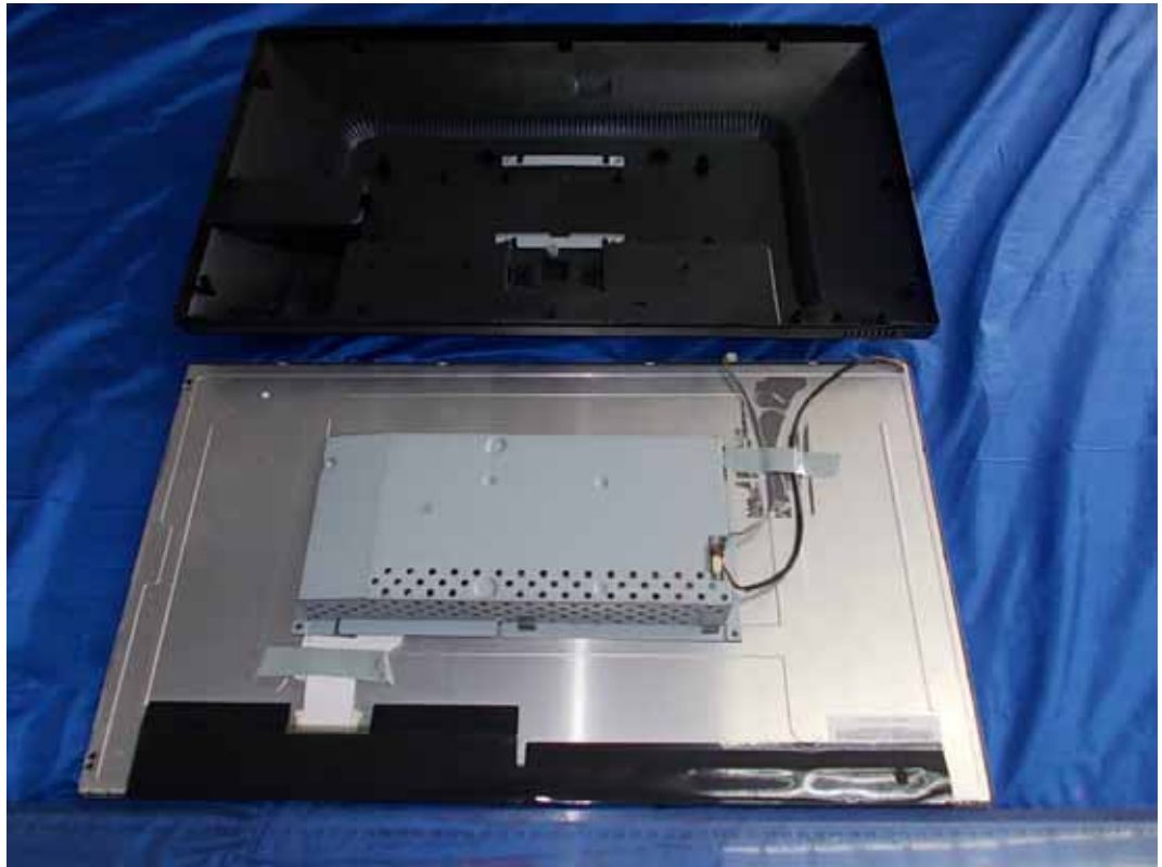
FIGURE 1 LCD MONITOR (M/N: E2411PX) COVER REMOVED
