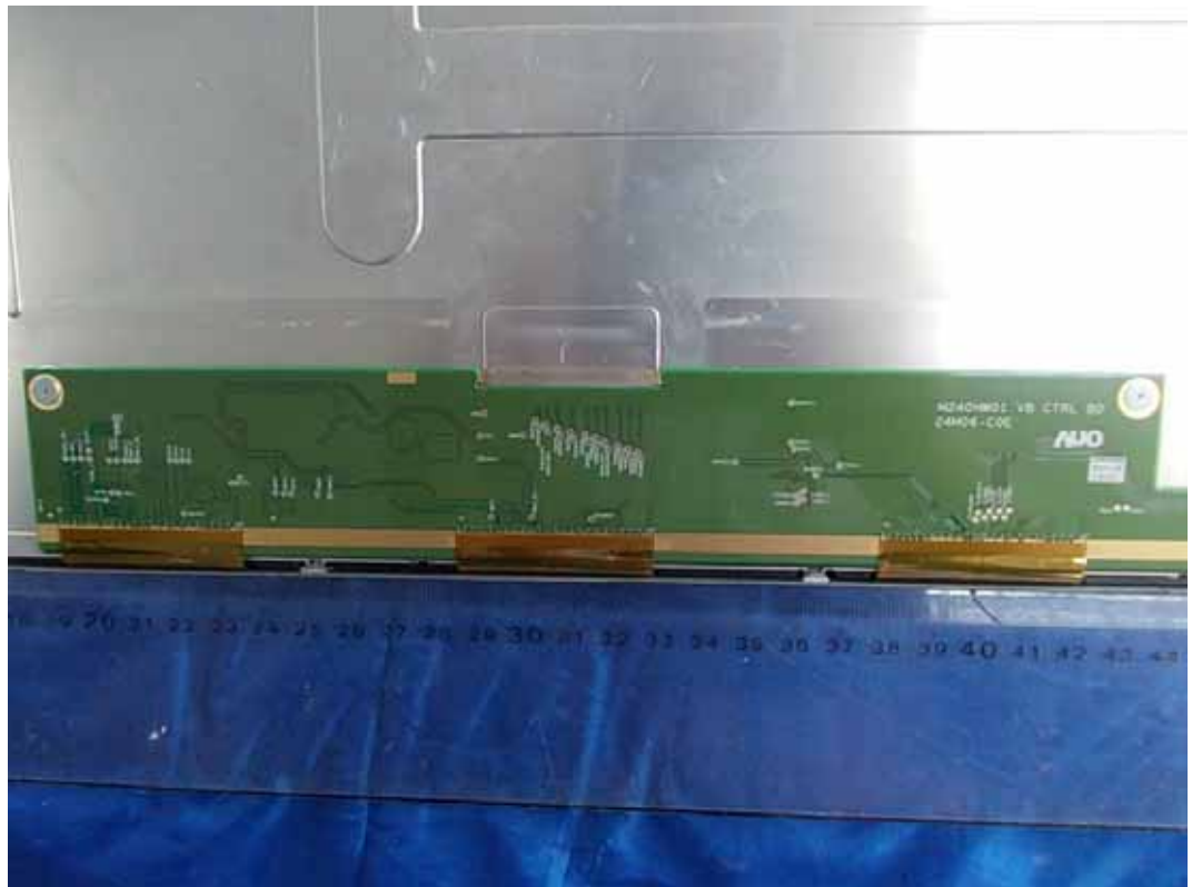
FIGURE 12 LCD MONITOR (M/N: E2411PX) LCD PANEL BOARD (SOLDERED SIDE-1)
