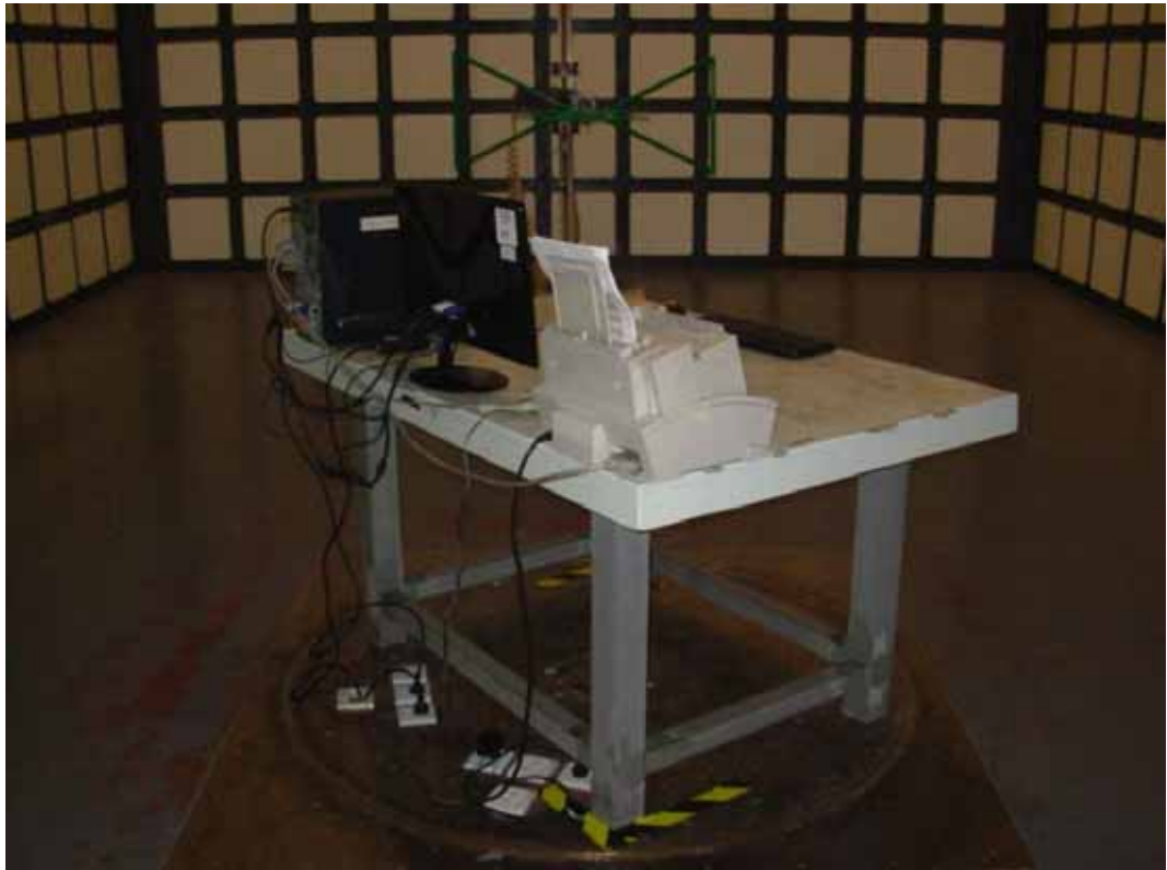
SETUP WITH MAXIMUM DETECTED EMISSION AT HORIZONTAL POLARIZATION (TEST MODE: DVI 1024*768@60Hz) (ADAPTER: DSA-36W-12 1 24)
