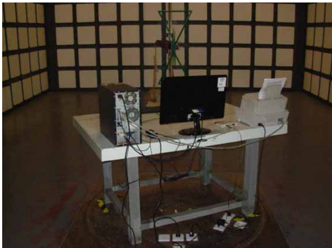
SETUP WITH MAXIMUM DETECTED EMISSION AT VERTICAL POLARIZATION (TEST MODE: DVI 1024*768@60Hz) (ADAPTER: DSA-36W-12 1 24)
