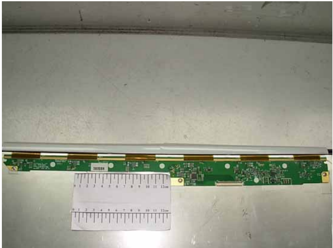
FIGURE 8 LCD MONITOR (M/N: E2250TV) LCD PANEL BOARD (COMPONENT SIDE)
