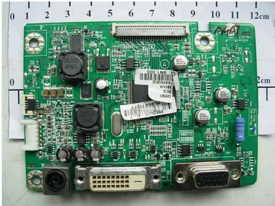
FIGURE 2 LCD MONITOR (M/N: E2250TV) MAIN BOARD (COMPONENT SIDE)
