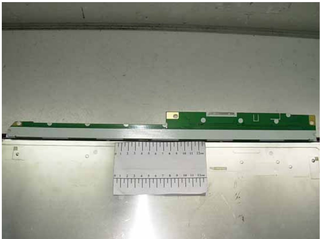
FIGURE 9 LCD MONITOR (M/N: E2250TV) LCD PANEL BOARD (SOLDERED SIDE)
