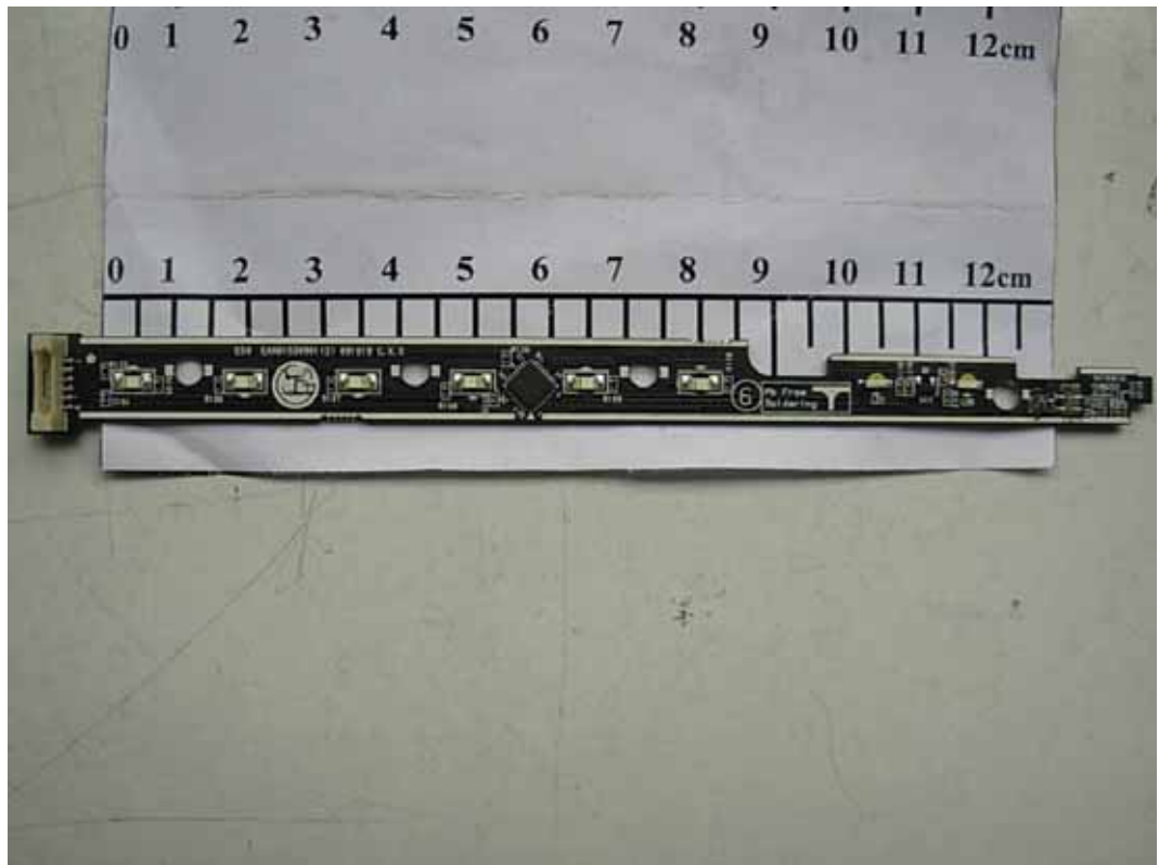
FIGURE 5 LCD MONITOR (M/N: E2250TV) KEY BOARD (COMPONENT SIDE)
