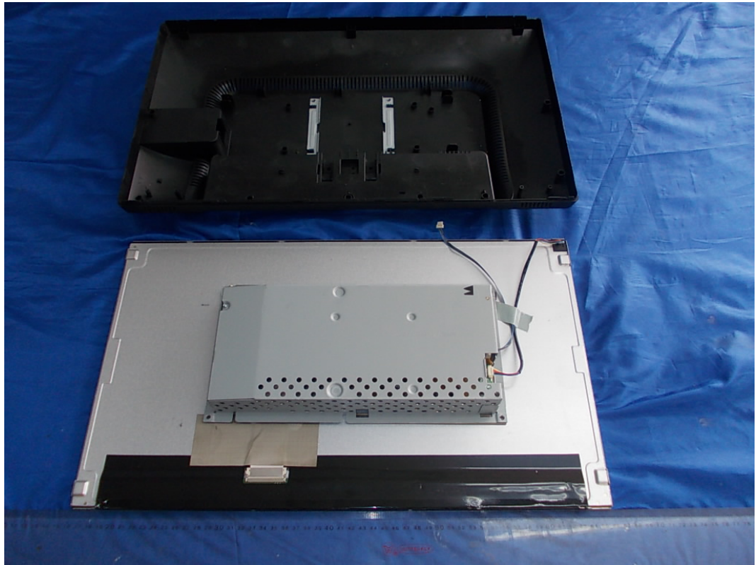
FIGURE 1 LCD MONITOR (M/N: E2211PX) COVER REMOVED
