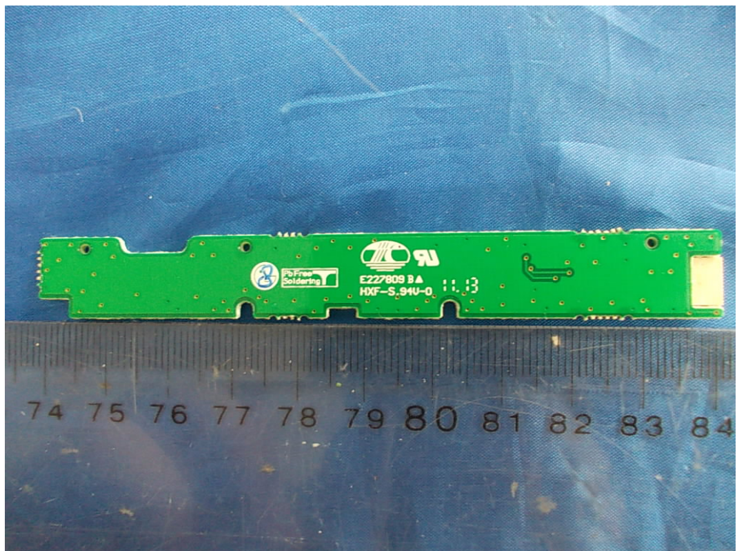
FIGURE 9 LCD MONITOR (M/N: E2211PX) KEY BOARD (SOLDERED SIDE)
