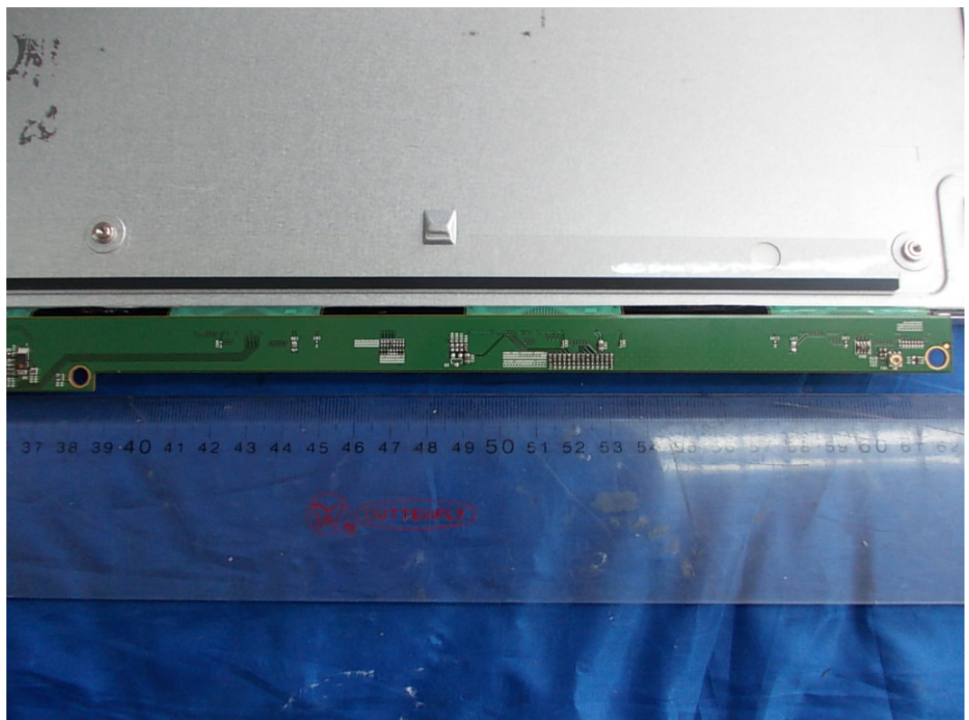
FIGURE 11 LCD MONITOR (M/N: E2211PX) LCD PANEL BOARD (COMPONENT SIDE-2)
