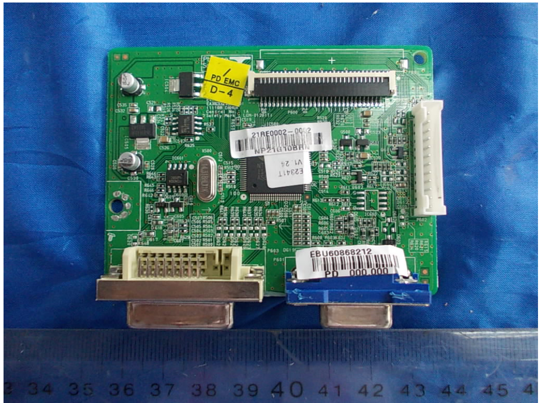
FIGURE 5 LCD MONITOR (M/N: E2211PX) MAIN BOARD (COMPONENT SIDE)
