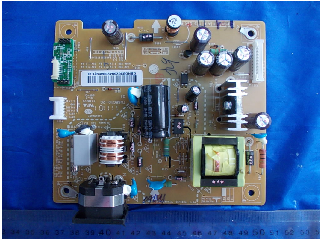
FIGURE 3 LCD MONITOR (M/N: E2211PX) POWER BOARD (COMPONENT SIDE)
