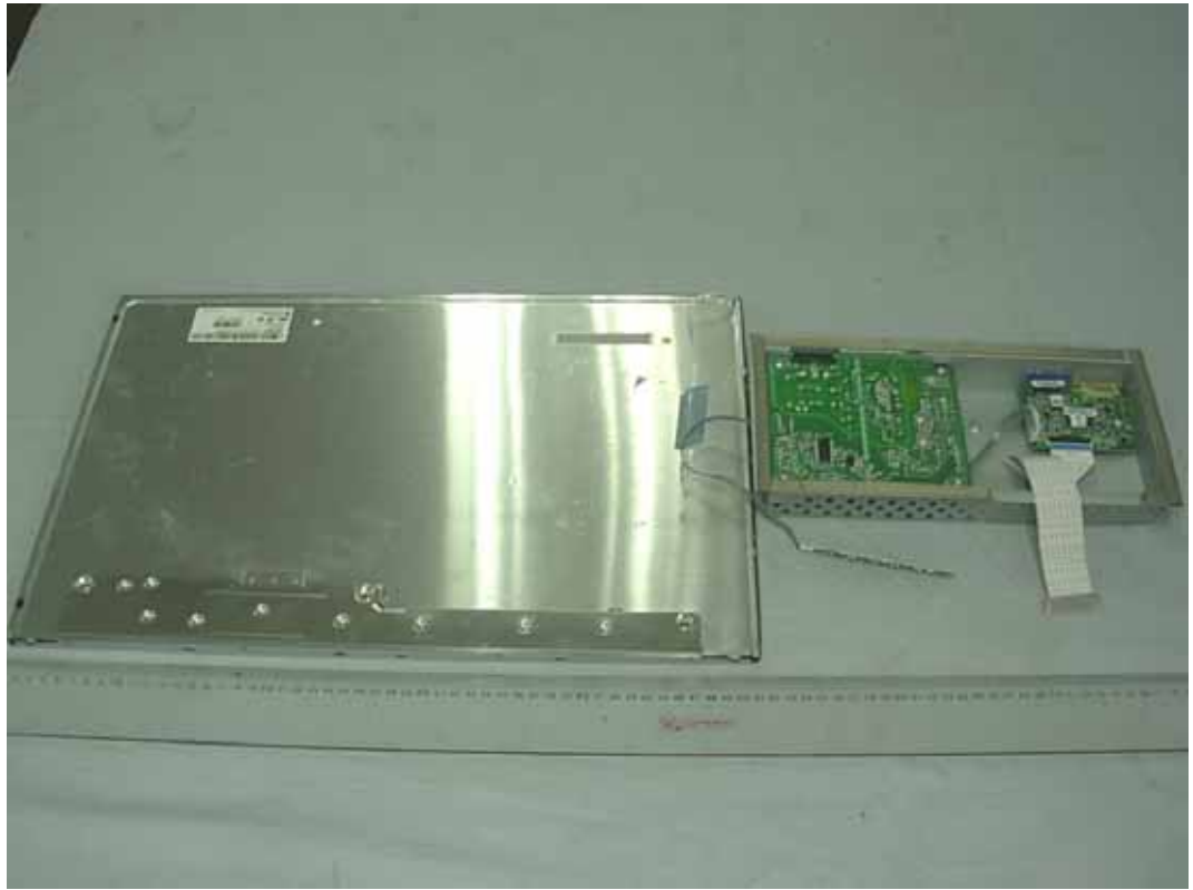
FIGURE 6 LCD MONITOR (M/N: E2210PW) BOARDS REMOVED
