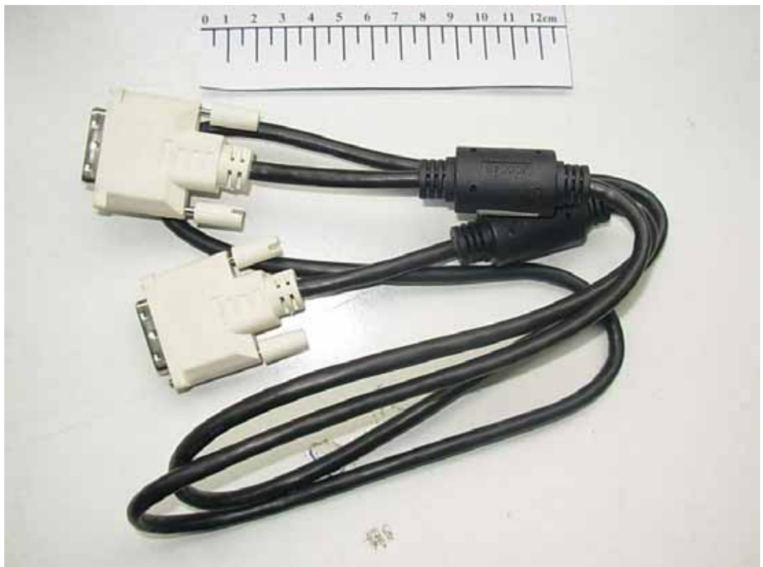
FIGURE 8 LCD MONITOR (M/N: E2210PMW) DVI CABLE #1
