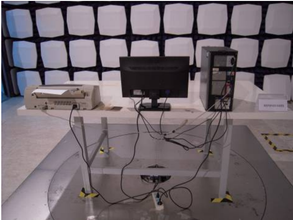
Back View of Radiated Emission Test
