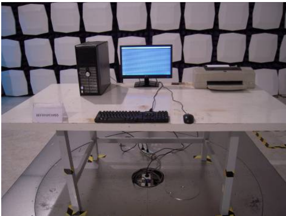
Front View of Radiated Emission Test
