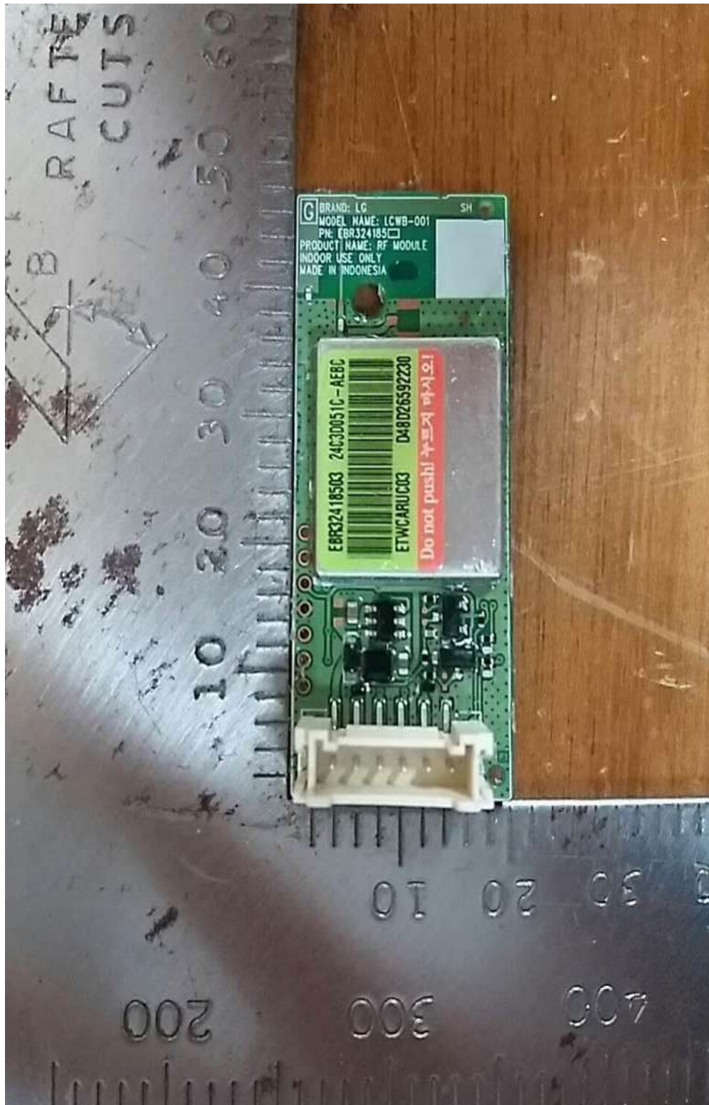
Alternated New Item_< Wi-Fi module Section -1>
