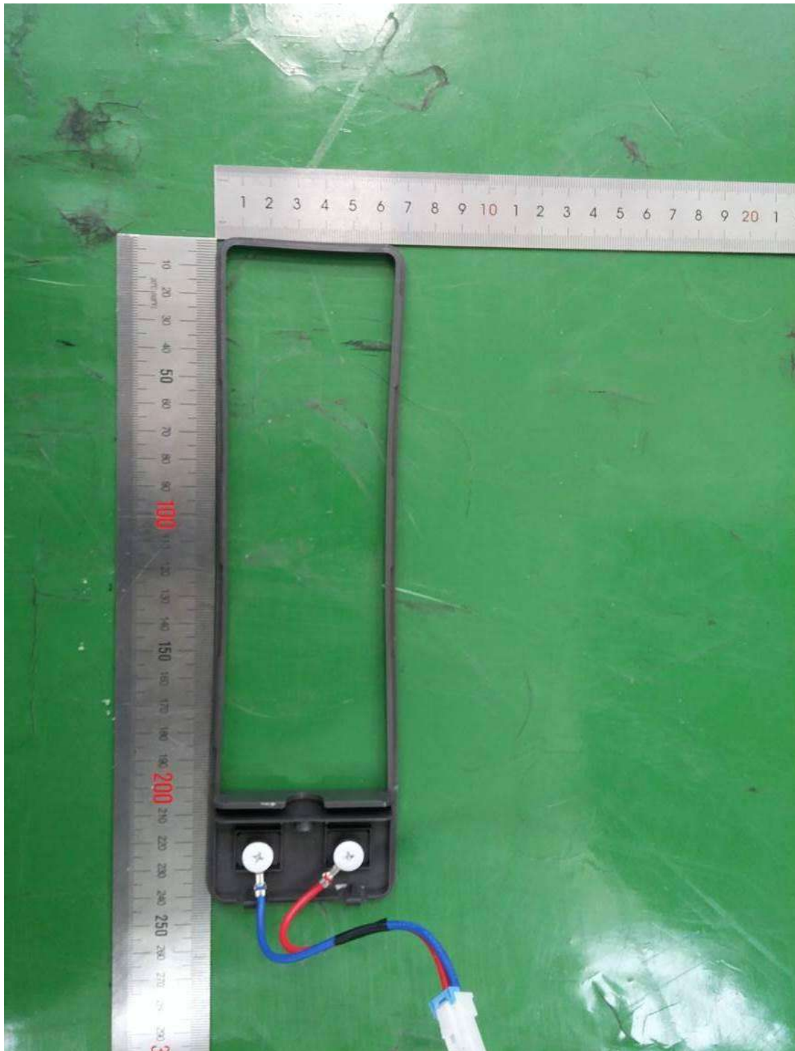
<Pillar Heater Section-1>
