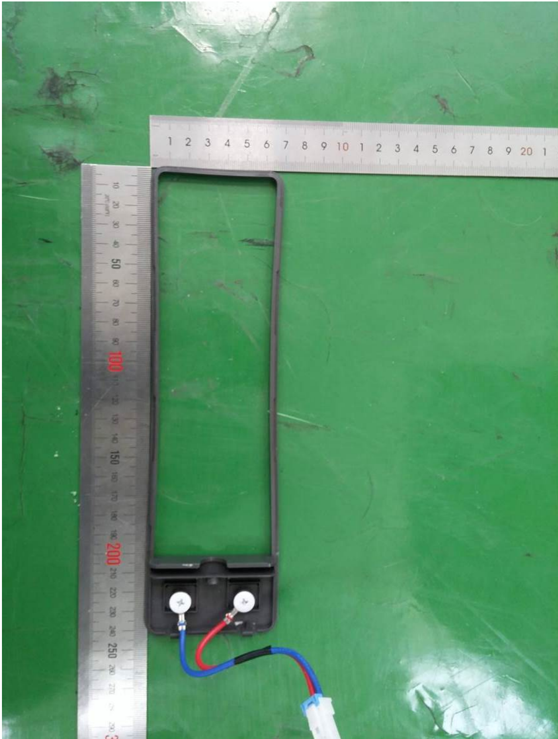
<Pillar Heater Section-1>
