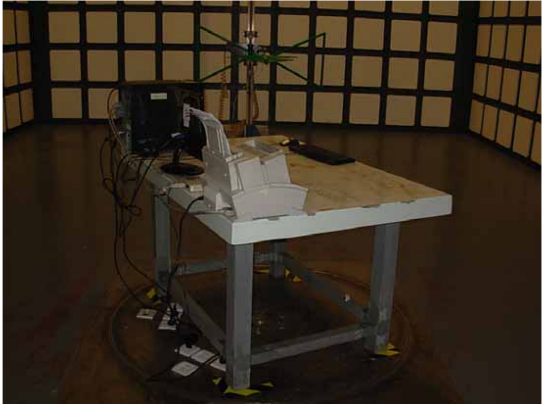
SETUP WITH MAXIMUM DETECTED EMISSION AT HORIZONTAL POLARIZATION (TEST MODE: DVI 640*480@60Hz) (ADAPTER: ADS-24NP-12-1 12024G)
