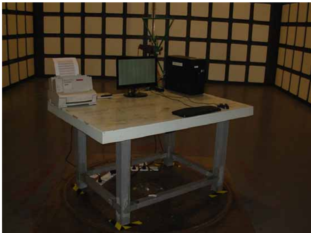
SETUP WITH MAXIMUM DETECTED EMISSION AT VERTICAL POLARIZATION (TEST MODE: DVI 640*480@60Hz) (ADAPTER: ADS-24NP-12-1 12024G)
