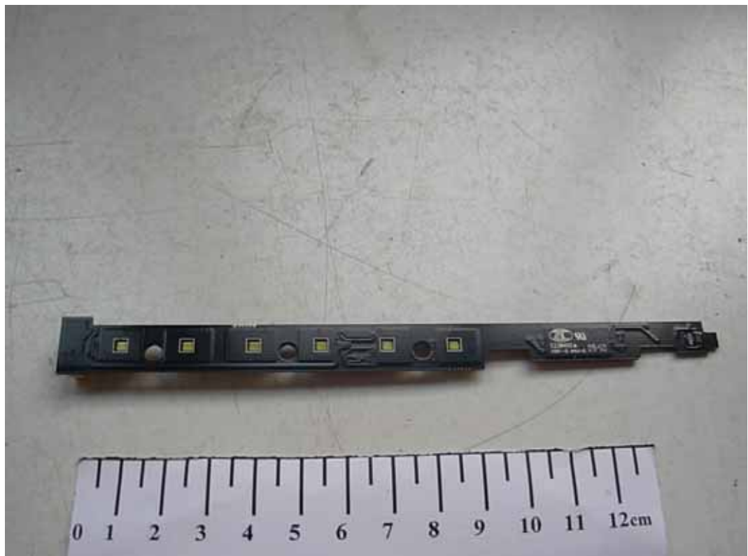
FIGURE 7 LCD MONITOR (M/N: E1950TV) KEY BOARD (SOLDERED SIDE)
