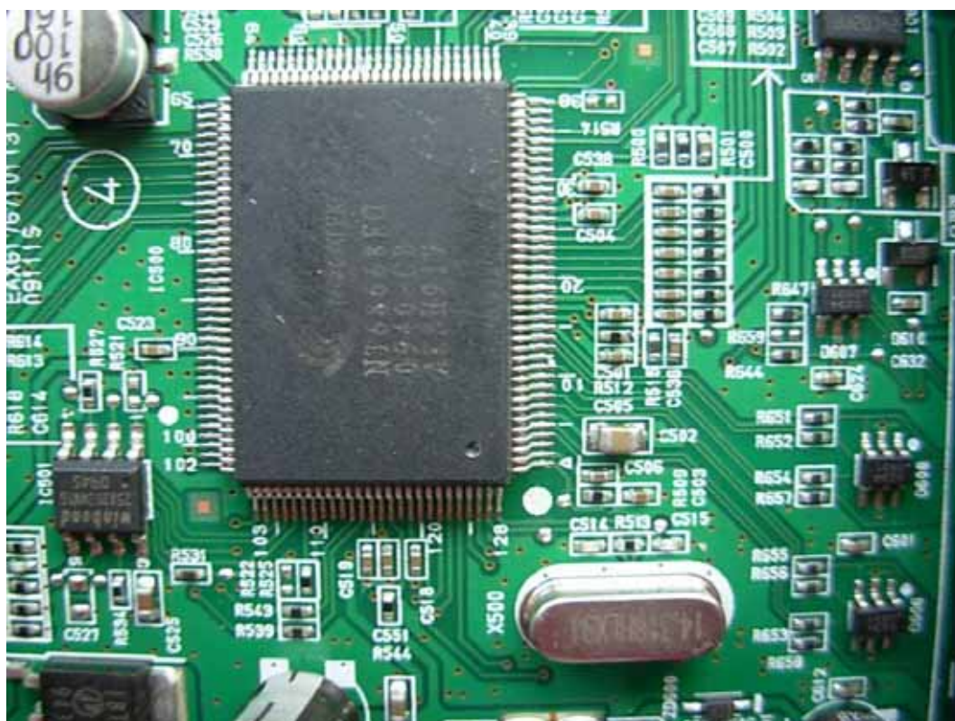
FIGURE 5 LCD MONITOR (M/N: E1950TV) CHIP & CRYSTAL ON MAIN BOARD
