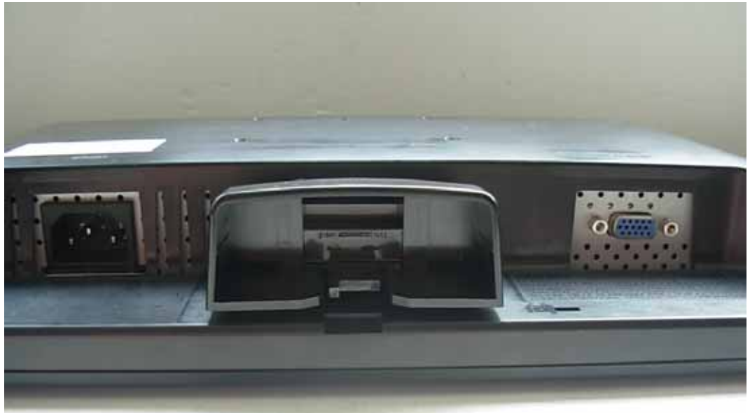
FIGURE 3 LCD MONITOR (M/N: E1641SX) SIGNAL PORTS & AC POWER PORT
