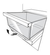
2 Keeping both levers pressed, lift the drawer support slightly and remove it from the rail system.
