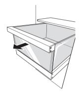
2 Lift the empty drawer slightly to remove it from the support.
