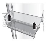
To replace the freezer door bin, align both sides of the bin with the guides and push the bin down until it snaps into place.
