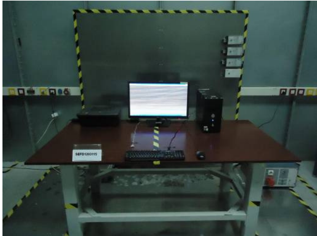
Back View of Conducted Emission Test
