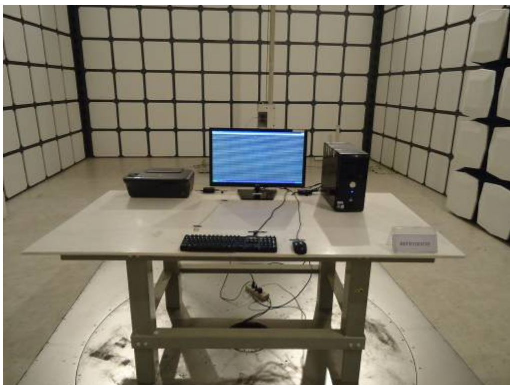
Front View of Radiated Emission Test (1000MHz ~ 18000MHz)
