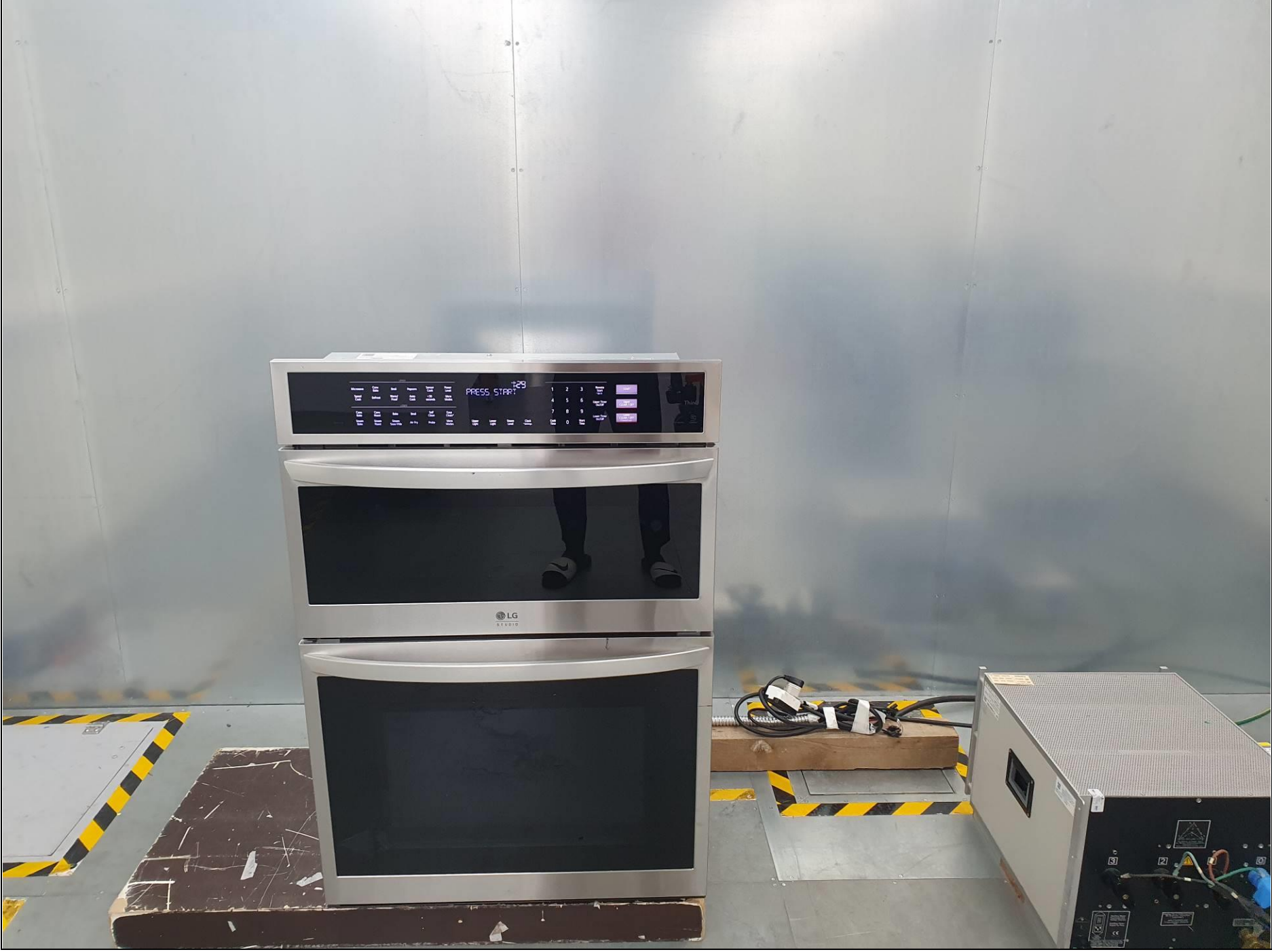
Continuous Conducted Emission at main _ Front
