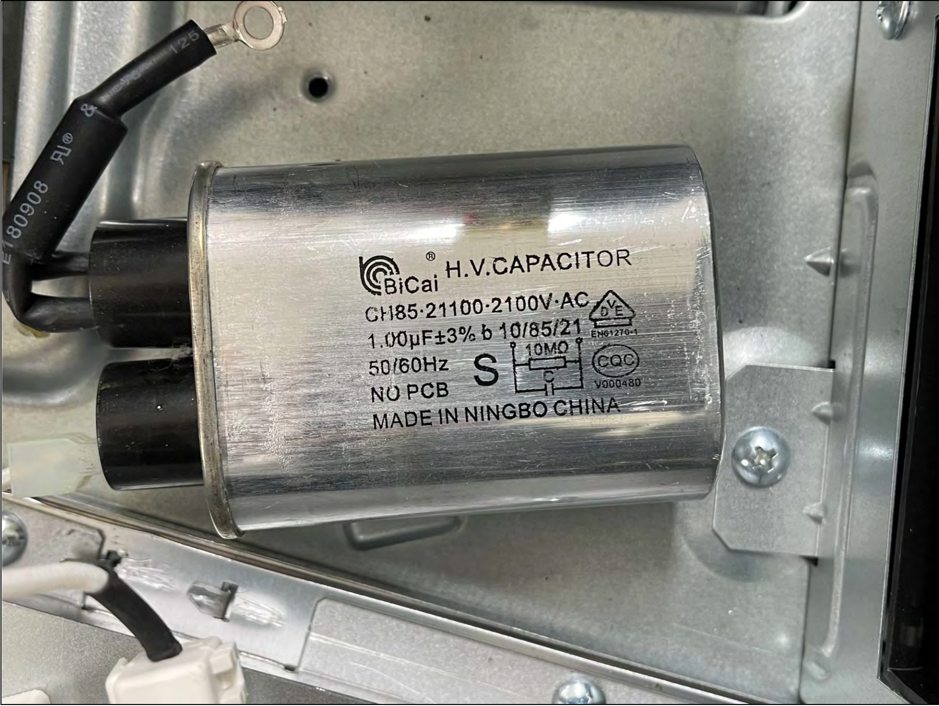
View of Capacitor
