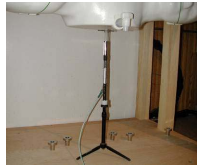
Figure 12-2 System Verification Setup Photo
