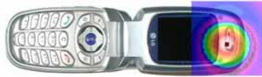
Figure A T-coil Location
