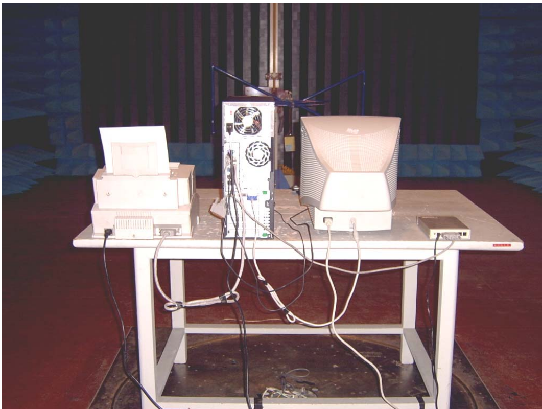
BACK VIEW OF RADIATED EMISSION TEST
