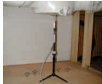
Figure 12.1 Dipole Validation Test Setup
