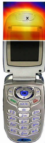
Figure 29 Sample E-field Scan Overlay
