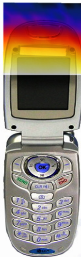
Figure 30 Sample H-field Scan Overlay
