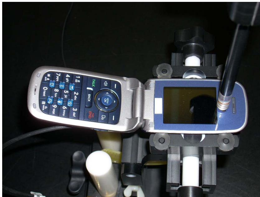
Figure 13-2 Test Setup for Wireless Device
