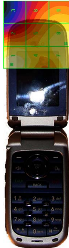
Figure 17-5 H-Field WD Scan overlay
