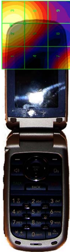
Figure 17-4 E-Field WD Scan overlay
