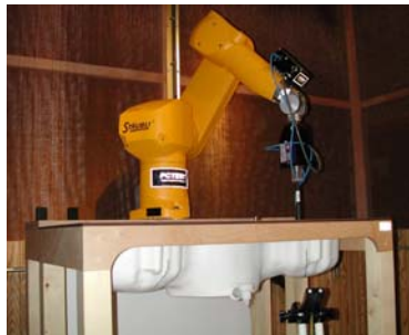
Figure 3-2 DASY4 SAR Measurement System
