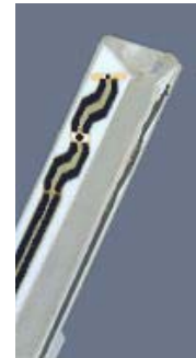
Figure 4-2 Probe Thick Film Technique
