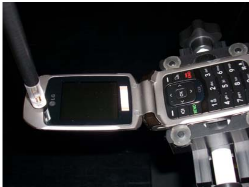
Figure 13-2 Test Setup for Wireless Device
