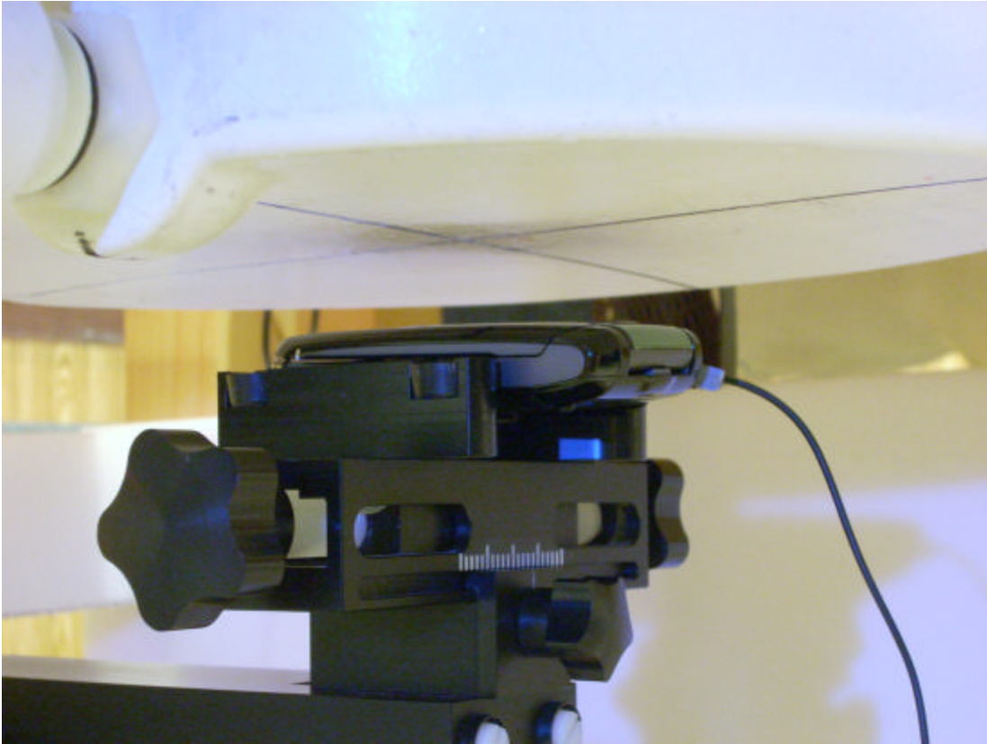
Figure 9: Body SAR, Front Side with 20mm Space
