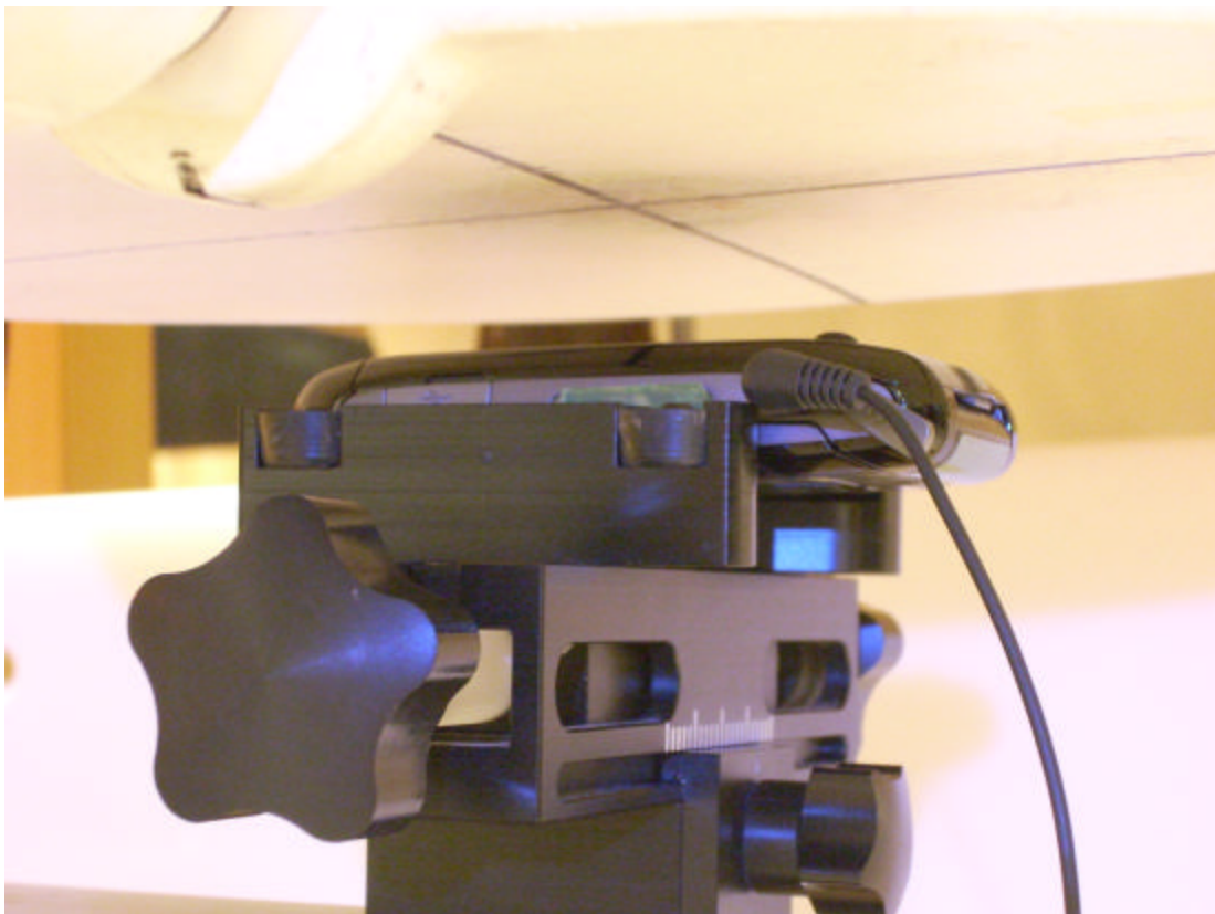
Figure 8: Body SAR, Back Side with 20mm Space
