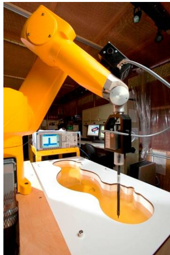
Figure 3-2 DASY4 SAR Measurement System
