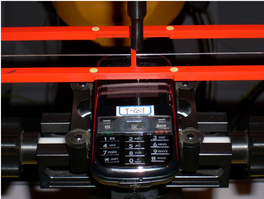
Figure 17-2 HAC Phantom Plane Alignment
