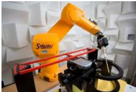
Figure 5-5 SPEAG Robotic System
