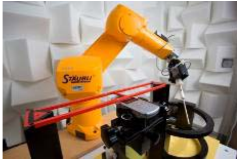
Figure 5-5 SPEAG Robotic System
