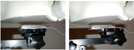
Figure 14.9 Body SAR Test Setup -- w/o Belt-clip --
