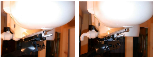
Figure 14.4 Left Head SAR Test Setup -- Ear / Tilt Position --
