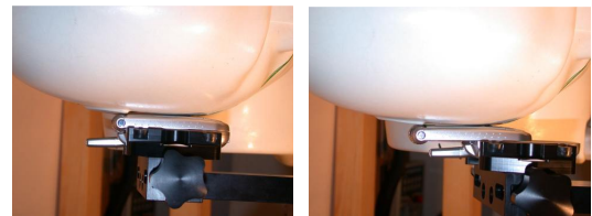
Figure 14.1 Right Head SAR Test Setup -- Cheek / Touch Position --
