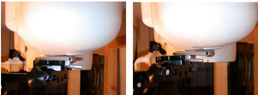
Figure 14.3 Left Head SAR Test Setup -- Cheek / Touch Position --
