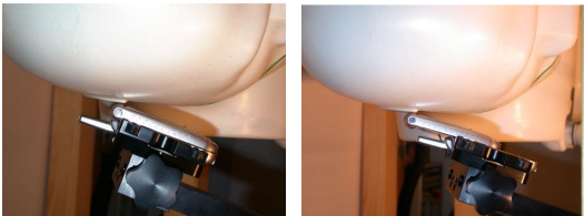
Figure 14.6 Right Head SAR Test Setup -- Ear / Tilt Position --
