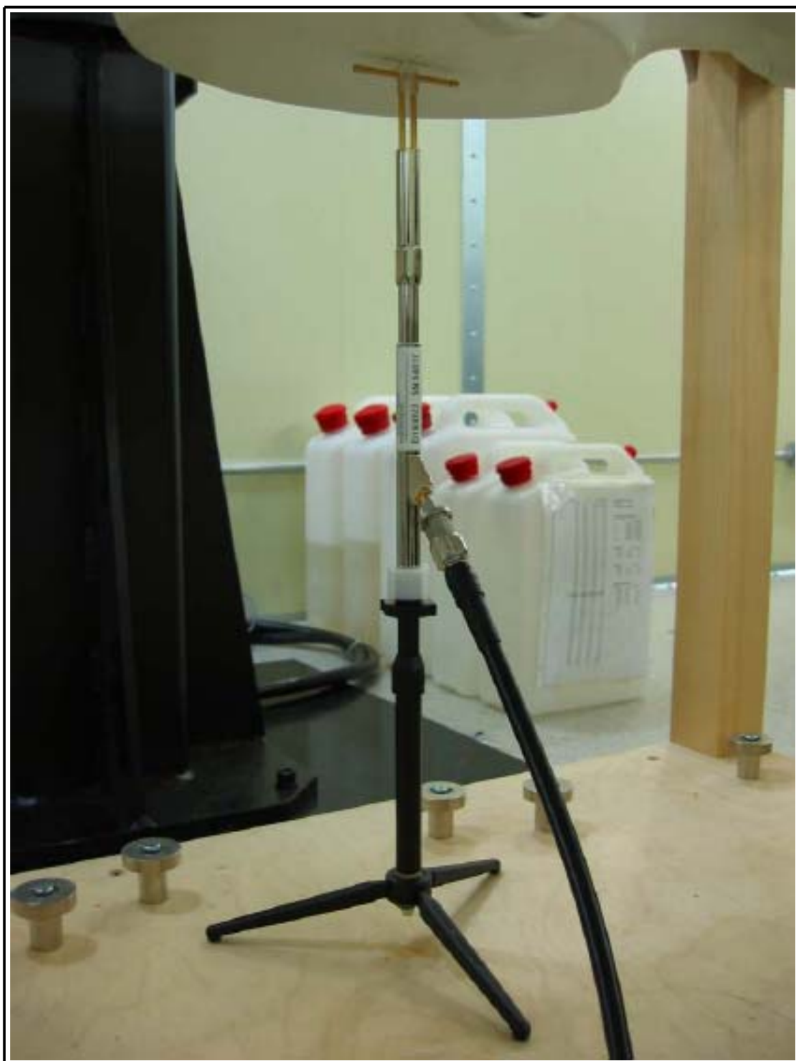
Figure 2 1900 MHz Dipole Validation Test Setup
