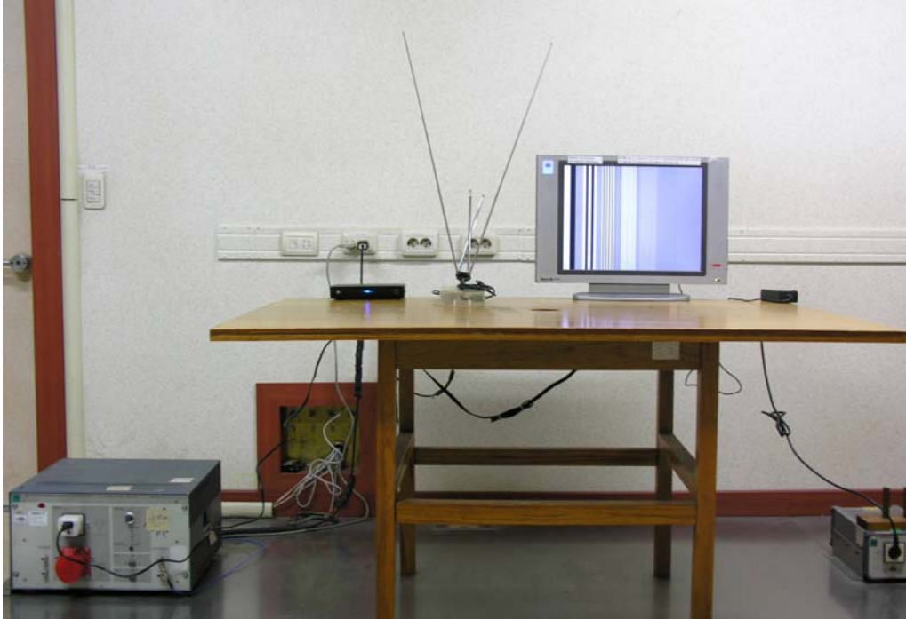
Photograph of Test Set-up (Power line conducted emissions)
