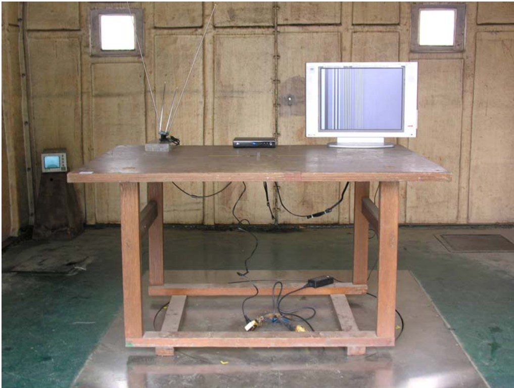
Photographs of Test Set-up (Radiated emissions)
