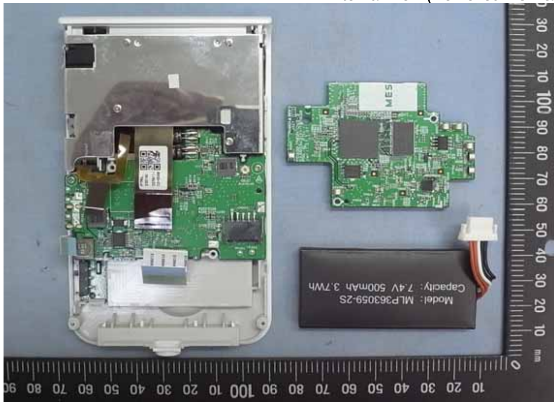
Figure 11 Internal View (Removed PCB & Battery)
