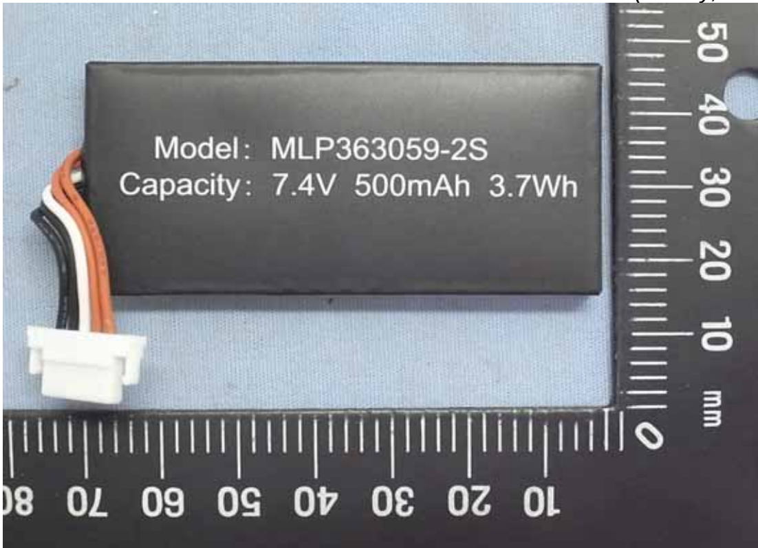
Figure 23 Internal View (Battery, Front View)
