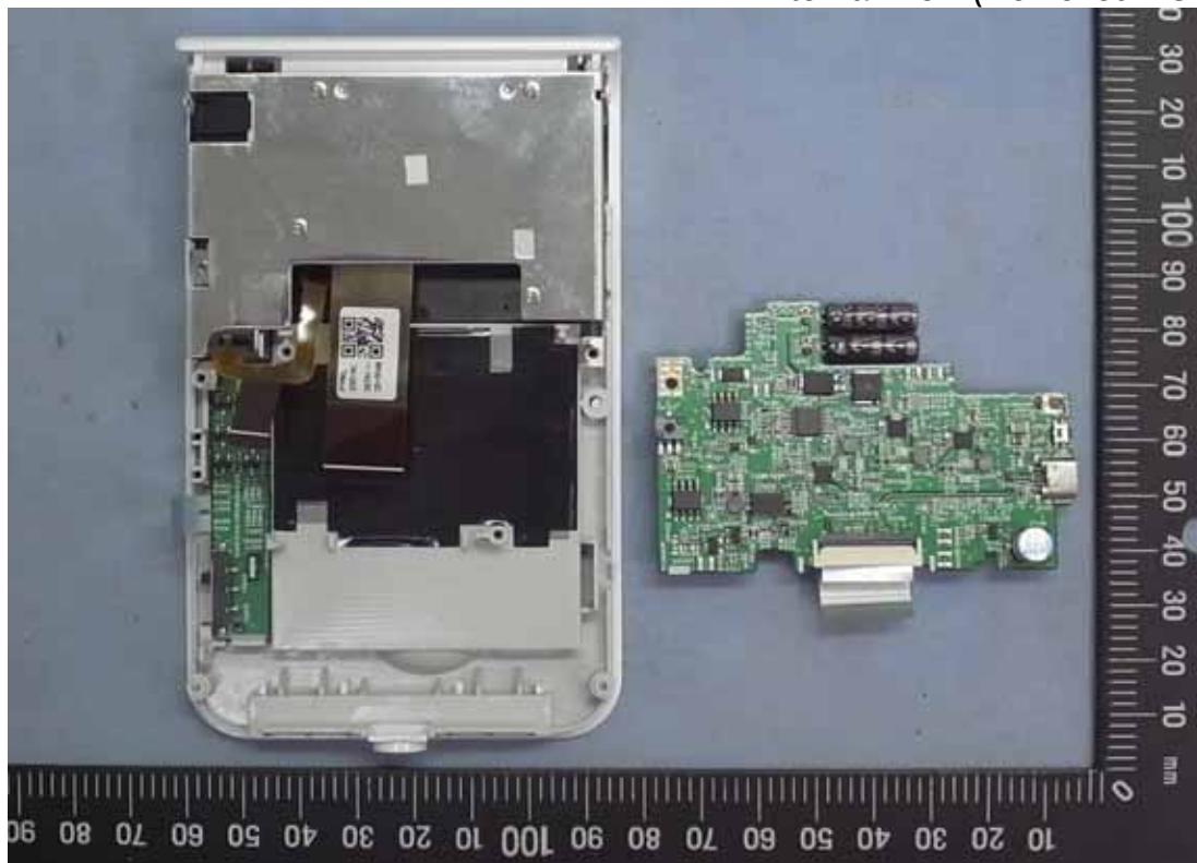
Figure 12 Internal View (Removed PCB Board)
