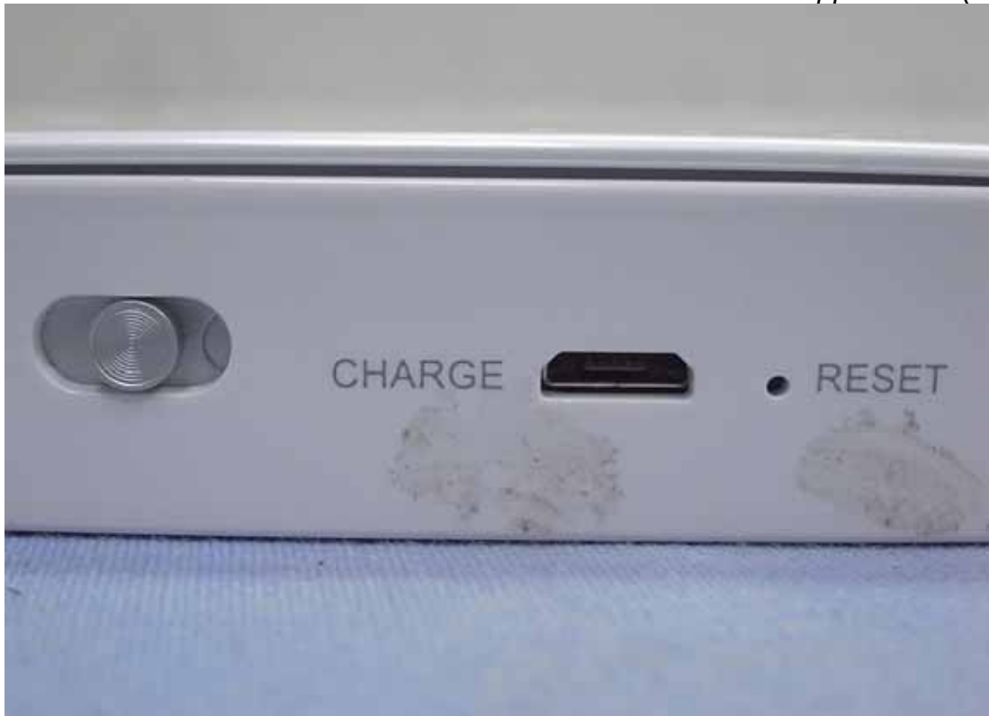
Figure 3 General Appearance (I/O Ports)
