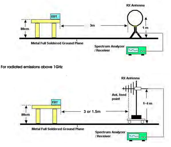
Above 5GHz shall be extrapolated to the specified distance using an extrapolation factor of 20 dB/decade from 3m to 1.5m.
