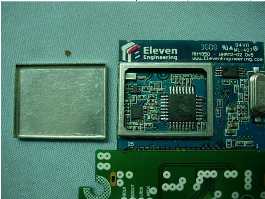
M/N HW904PA, Internal View (RF Module Board, Front View)
