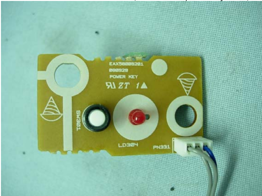
Figure 58 M/N HW964TZ, Internal View (Power Key Board, Front View)
