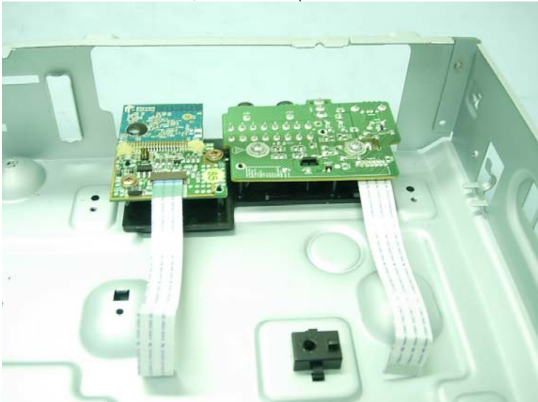
Figure 62 M/N HW964TZ, Internal View (RF Module Board & USB/PTB/MIC Board)
