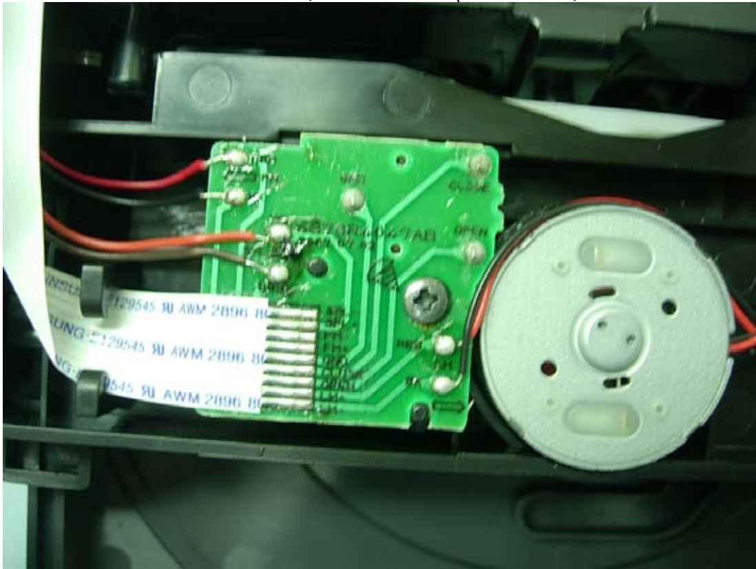
Figure 21 M/N HW904PA, Internal View (DVD Driver, Control Board/Back View)
