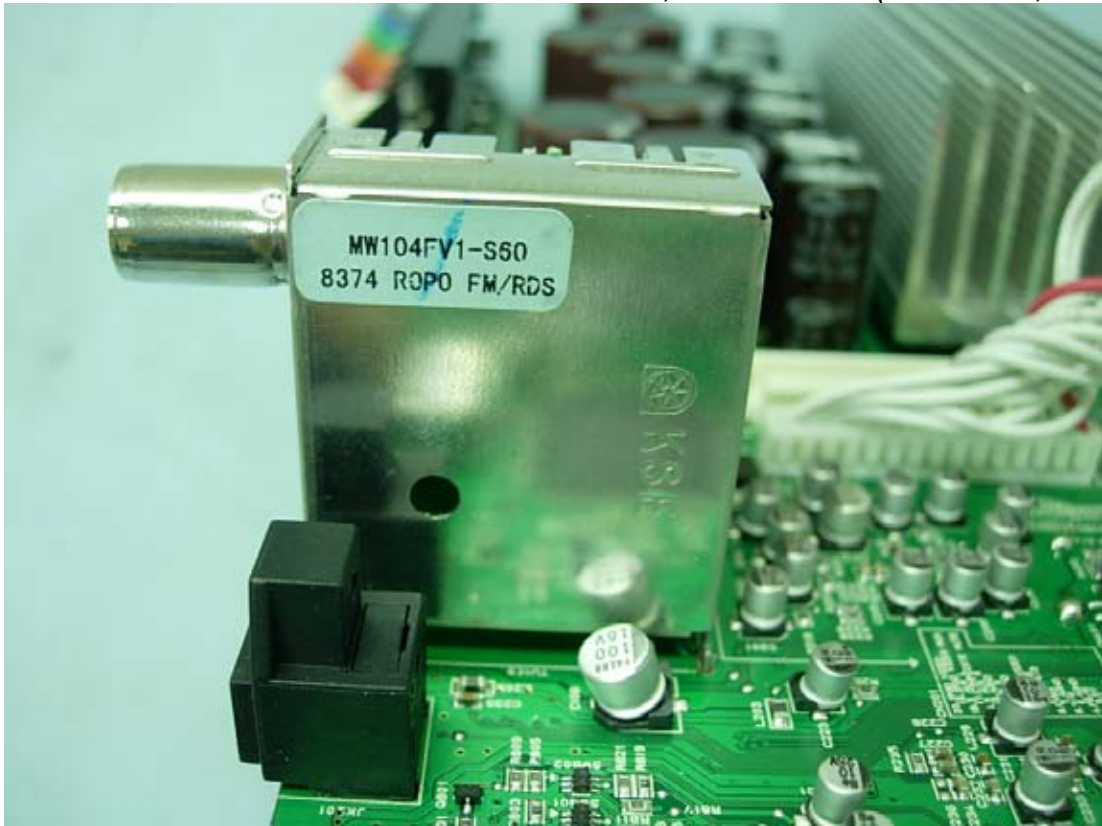
Figure 47 M/N HW964TZ, Internal View (Tuner Unit, Front View)
