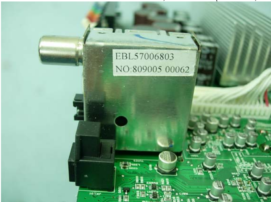
Figure 16 M/N HW904PA, Internal View (Tuner Unit, Front View)
