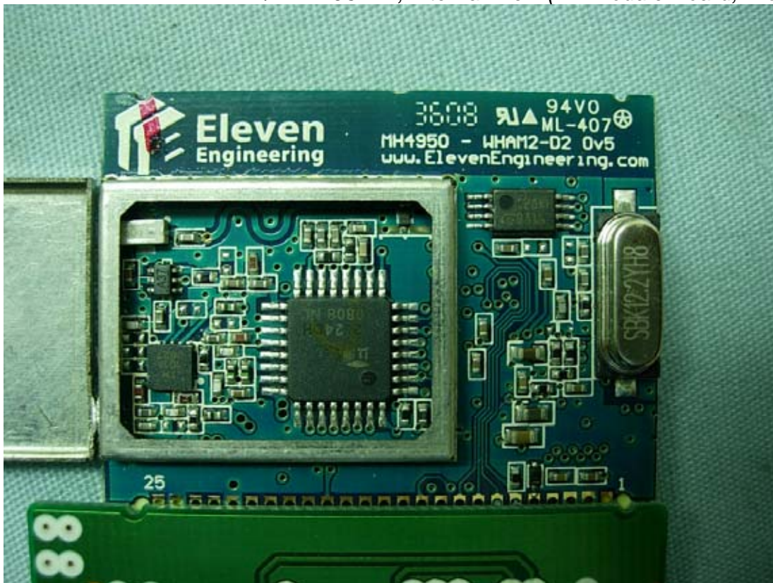
Figure 66 M/N HW964TZ, Internal View (RF Module Board, Front View)
