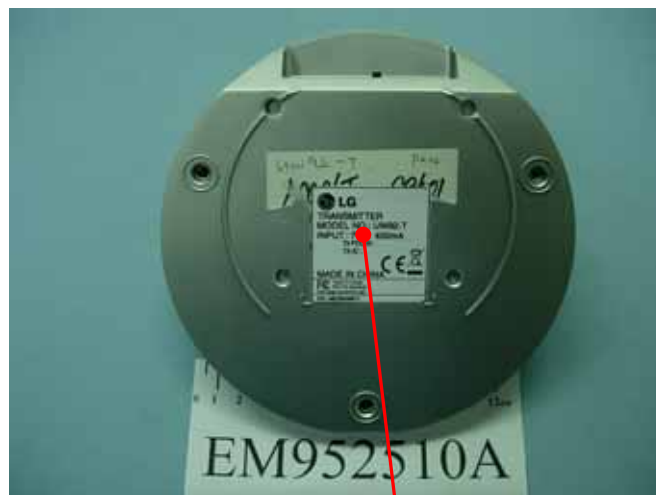
FCC Label Placement Location
