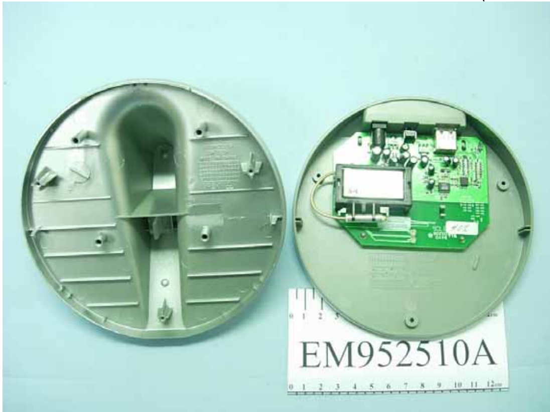
Figure 4 Internal View (Removed Cover)
