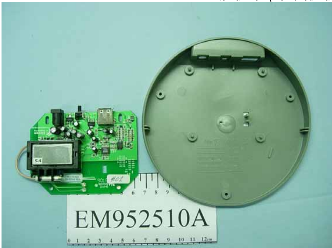
Figure 5 Internal View (Removed Main Board)
